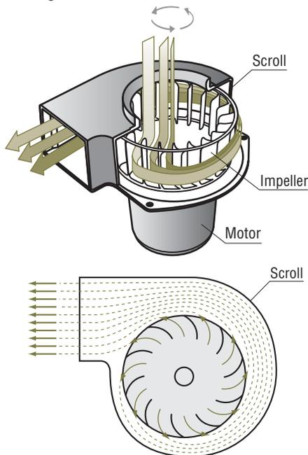
Fig. 2 Structure and Air Flow Mechanism of Centrifugal Blowers
